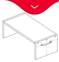
5. Select a desired handle position and mark with a pencil where fasteners will need to be inserted. Repeat for the opposite side.
