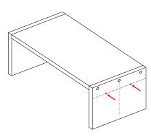
6. Drill a 3mm pilot hole for all fastener positions. Note: If your handles are secured from the outside, the pilot holes only need to be drilled half way through the timber thickness.
