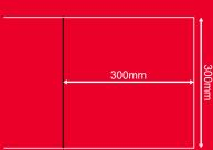
2. Measure & mark a 300mm square on the timber work piece. Clamp securely and cut along the line using a circular saw.
