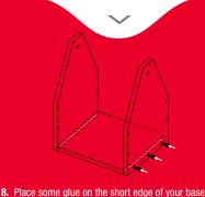
panel then align with the lower edge of the side panel. Use 40mm screws to secure together. Repeat for the opposite side.
