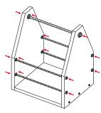
12. Secure rods by screwing the dome nuts onto the rod ends and then tightening the hex nuts so that the timber is sandwiched between.
