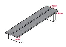
**6.** Place two decking boards with a 10mm gap onto two 190mm timber pieces so they over-hang 50mm both ends.
