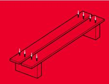
Fasten the decking boards down using 50mm screws. Create two of these seats. Note: Make sure to drill pilot holes and countersink prior to driving screws in.
