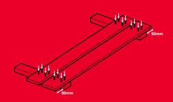
Place two decking boards with a 10mm gap onto two 410mm timber pieces so they over-hang 50mm both ends Fasten together using 50mm screws. Create two of these back rests
