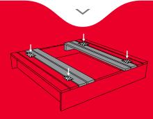
Place your two created seats into position with a 10mm gap between the secured decking boards. Attach two hinges to each seat using eight 20mm screws in each hinge.
