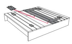
10. Place one back rest into position with a 10mm gap between the secured seats. Attach two hinges from the under-side using eight 20mm screws in each hinge.
