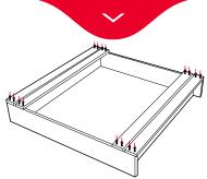
5. Fix in position using two 50mm screws at each end of the decking boards. Note: Prior to driving screws in, you should always drill pilot holes with a 3mm drill bit and countersink bit to prevent timber from splitting.
