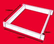
**4.** Place two decking boards at each end of the box with a 10mm gap between boards.
