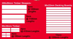
Clamp the timber securely and cut along your marks with the circular saw. You should now have all pieces shown above.
