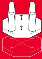
**9.** Align the 2 hexagon pieces so that the nuts go into the drilled holes. Then secure together by driving 4 screws between the legs.
