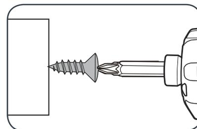
5 Lightly squeeze the variable speed trigger to start the driver.
