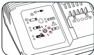
3 With the charger sitting on a flat surface, align the raised ribs on the battery with the recess in the charger and slide onto the charger ensuring a firm connection.
