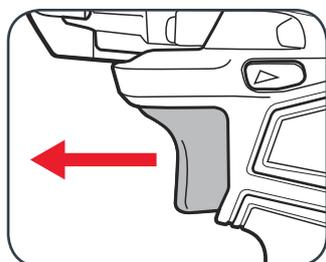
3 Control the speed by adjusting the amount of pressure applied to the trigger.
