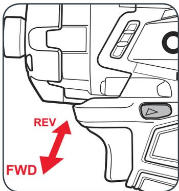
2 To remove screws and bolts, push the fwd/rev lever hard right.
