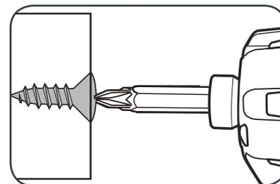
**Note:** Do not force the driver or apply side pressure to elongate the hole. Let the impact driver do the work.
