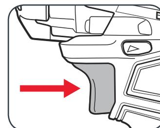
6 Slowly increase pressure on trigger to appropriate torque for circumstances until screw or bolt is tightened.
