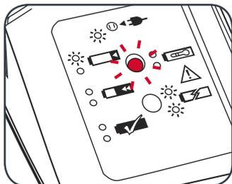
5 The charger LED will illuminate green once the battery is fully charged.
