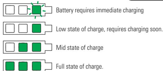
**Note:** The battery needs to be removed from the tool to check the state of charge.
